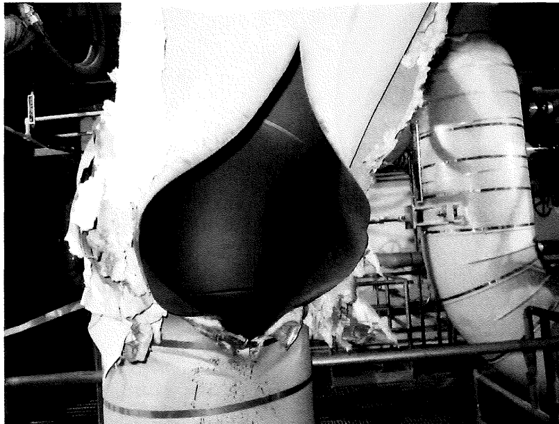
Photograph 2, Ruptured HP Turbine Exhaust pipe (South Leg)
