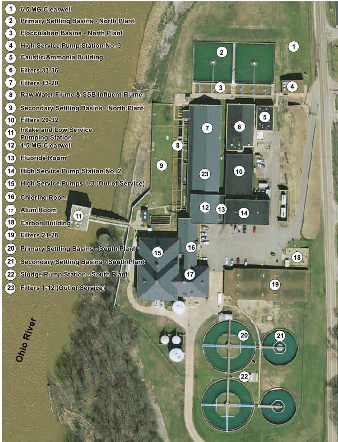
FIGURE 3-1 Site Plan of the Water Treatment Plant
