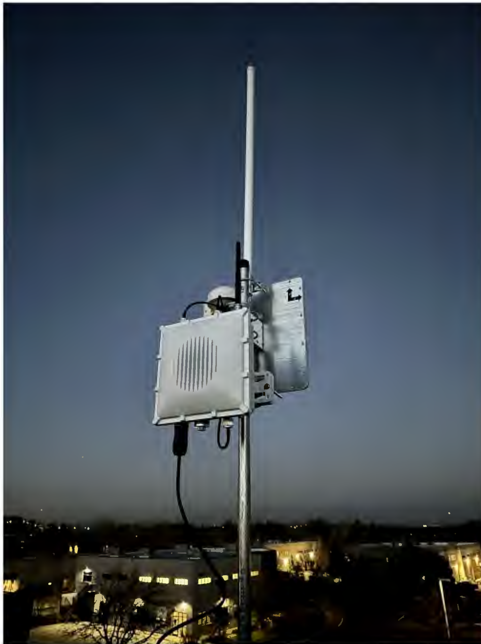
Copper Labs' neighborhood-level detector can remotely access data from hundreds of existing meters at once. Image courtesy Chris Choi.
