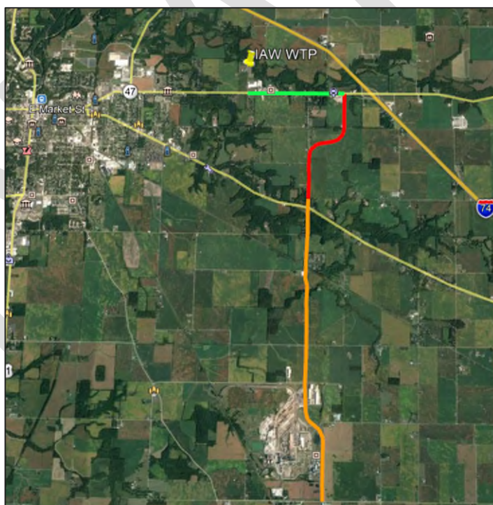
Figure 1. Proposed Installation of the New CRW Transmission Main (Phase 1 - green, Phase 2 - red, Phase 3 - orange)
