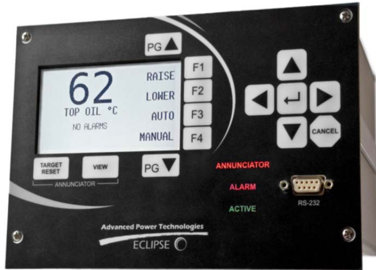
Figure 1. Display of monitor that is connected to SCADA RTU
