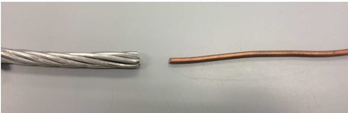
Figure 2. Aluminum conductors (left) became the industry standard approximately 30 years ago. This program focuses on replacing outdated conductors (such as the copper conductor on the right) to enhance safety, reliability, and capacity.
