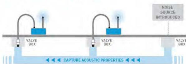
FIGURE 3: EPULSE® FOR DISTRIBUTION & TRANSMISSION MAINS ABOVE ILLUSTRATES THE TYPICAL FIELD SETUP FOR AN EPULSE FIELD MEASUREMENT.
