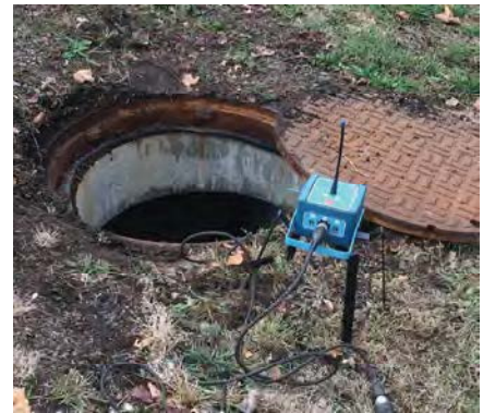
EPULSE® TECHNOLOGY DIDN'T REQUIRE AND EXCAVATION TO ACCESS THE WATER MAIN WHICH WAS CRITICAL FOR THIS PROJECT.
