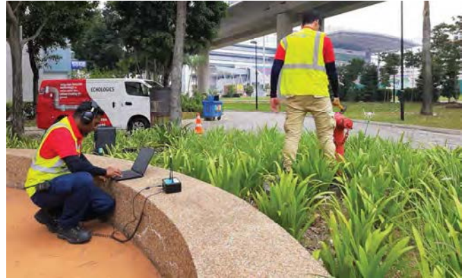
FIGURE 2: ECHOLOGICS FIELD SPECIALISTS GATHERING ACOUSTIC PROPERTIES OF A PIPE SEGMENT USING A LEAKFINDERST CORRELATOR
