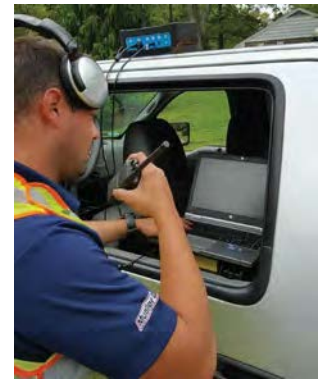
ECHOLOGICS FIELD ENGINEERS ASSESS THE CONDITION OF DUCTILE IRON PIPE
