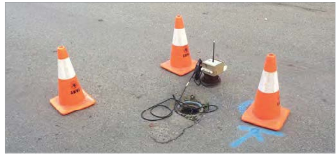
EPULSE® CONDITION ASSESSMENT TECHNOLOGY IS NON-INVASIVE AND SEARCHES FOR LEAKS SIMULTANEOUSLY.
