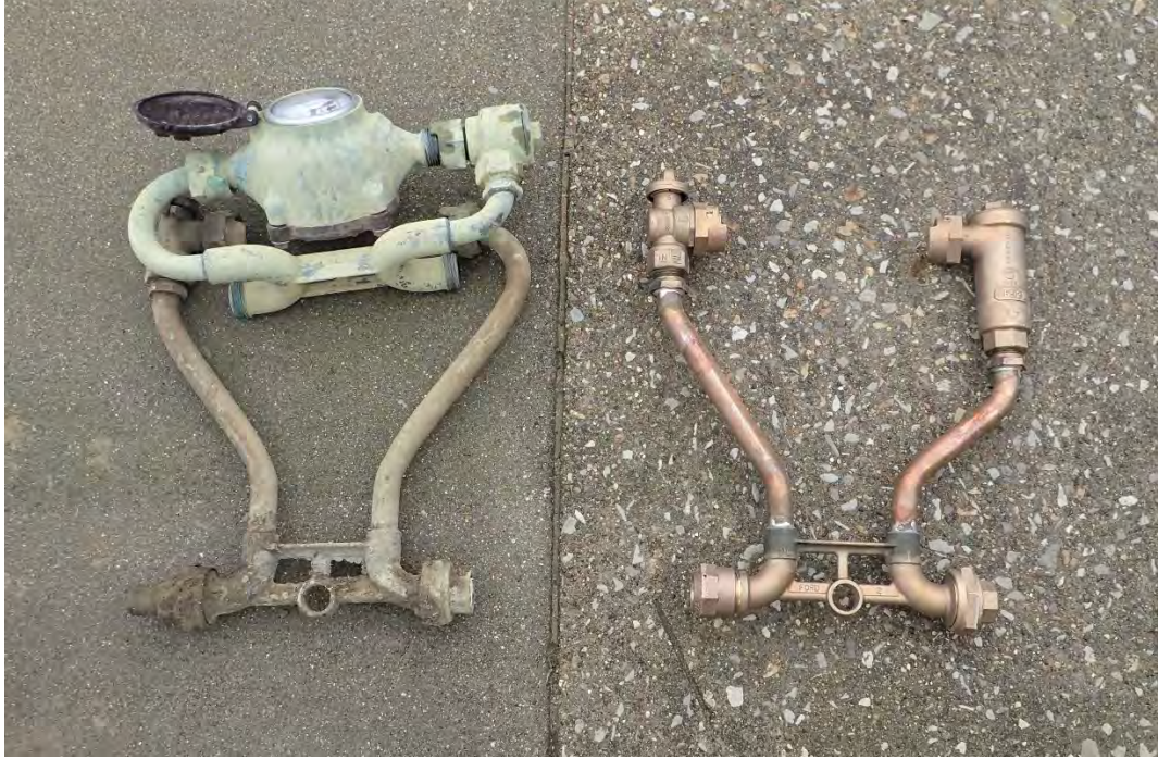
On left, sample meter setter to be replaced with unit with check valve on right
