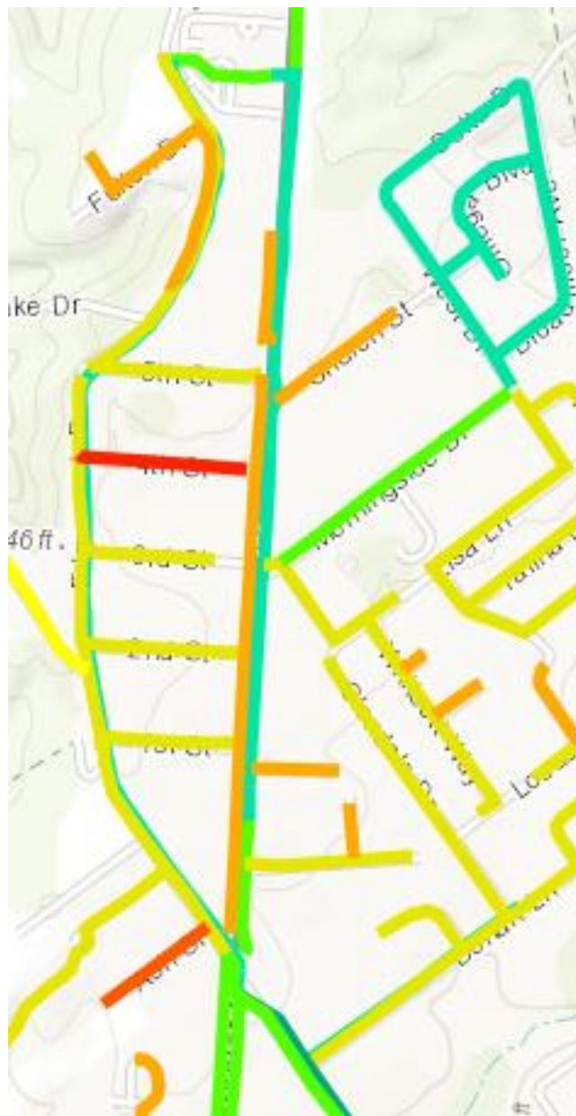
Figure 4 2016 Water System Map. All lines east of SR 3 are incorrectly listed as 2003 vintage. All lines west of SR 3 are incorrectly listed as 1978 vintage. The aqua colored line along SR 3 is correctly shown as 1967.
