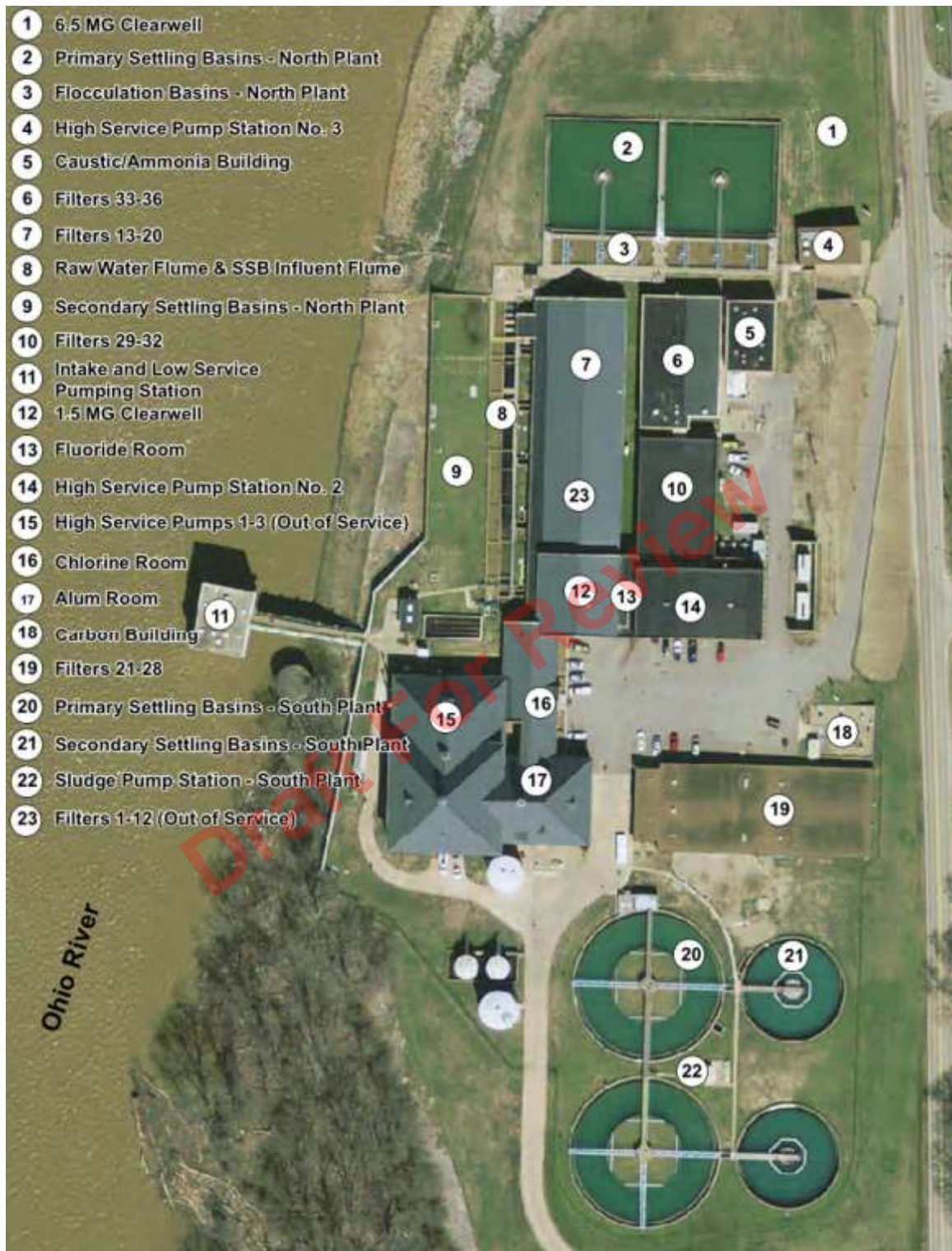
FIGURE 1-1 Site Plan of the Water Treatment Plant
