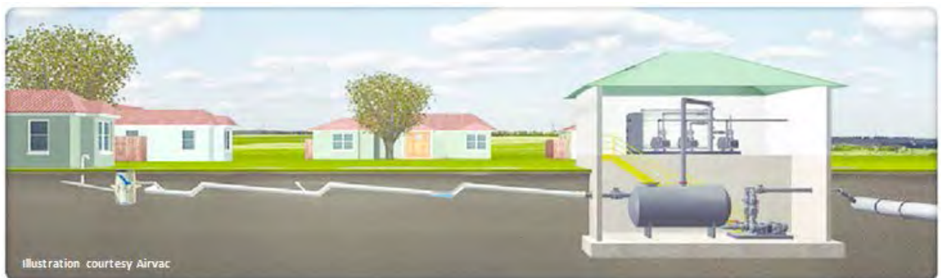
Figure 2 Typical Schematic of a Vacuum Sewer System
