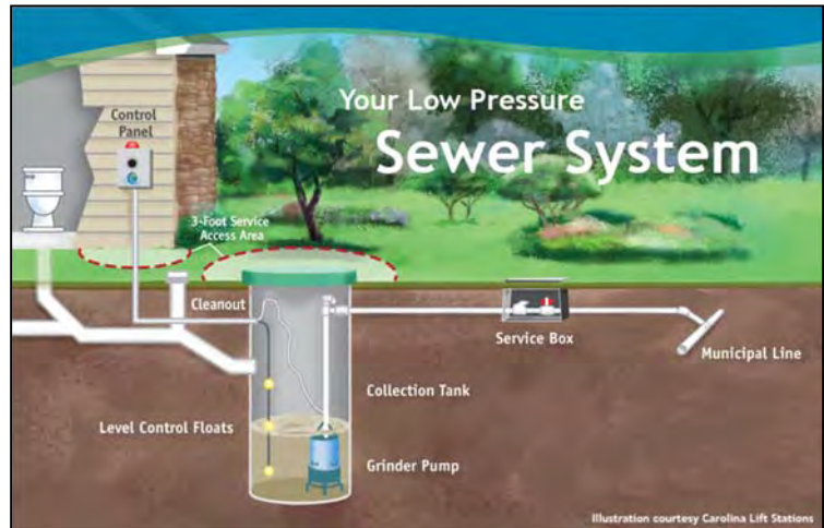
Figure 2: Typical Low Pressure System
