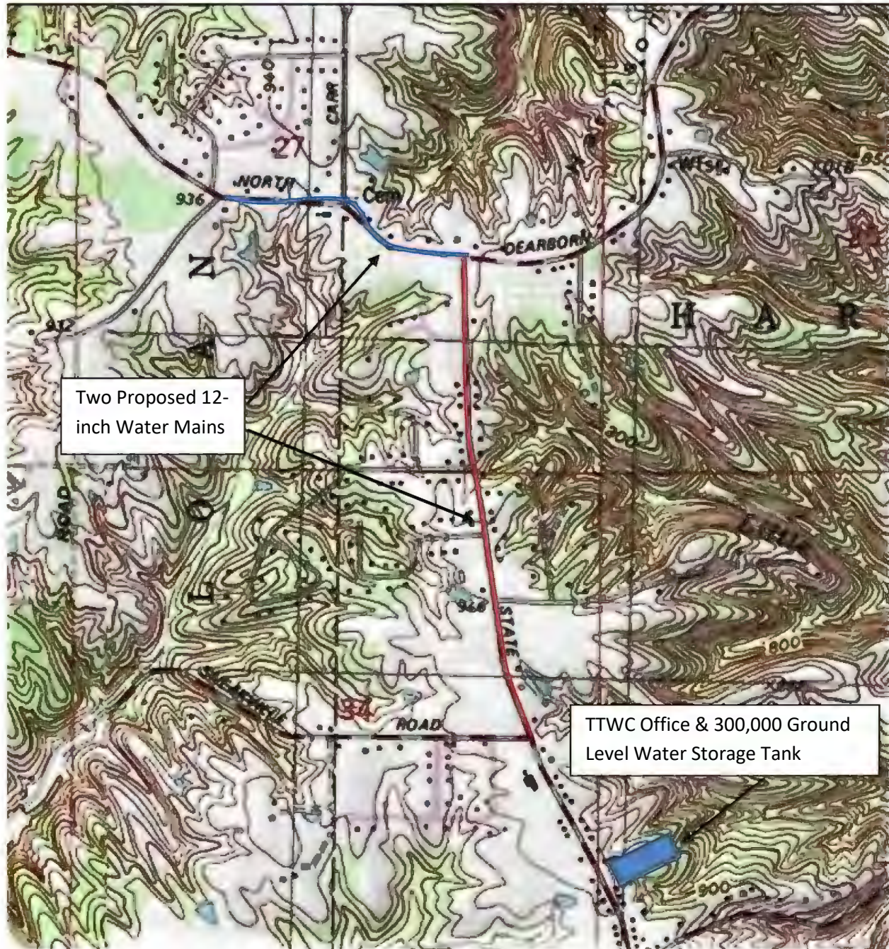
Figure 1.2.3 Location of Proposed 12-inch Water Main
