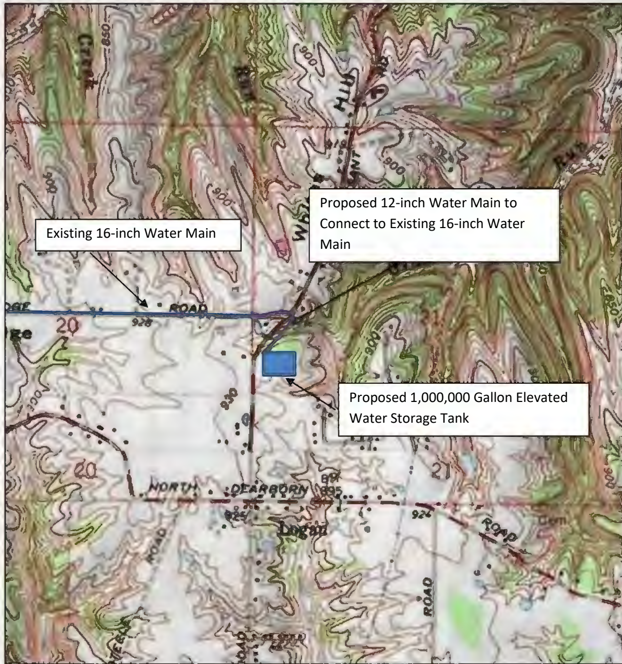
Figure 1.2.1 Location of Proposed Water Storage Tank
