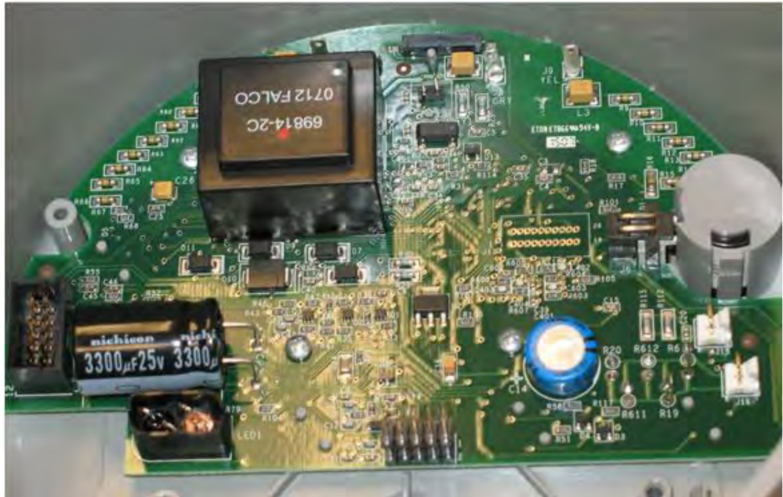
Meter board inside housing
