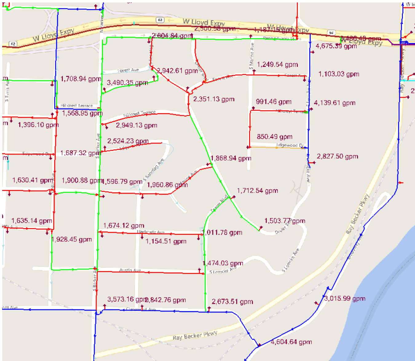
Figure 2. Existing Available Fire Flow
