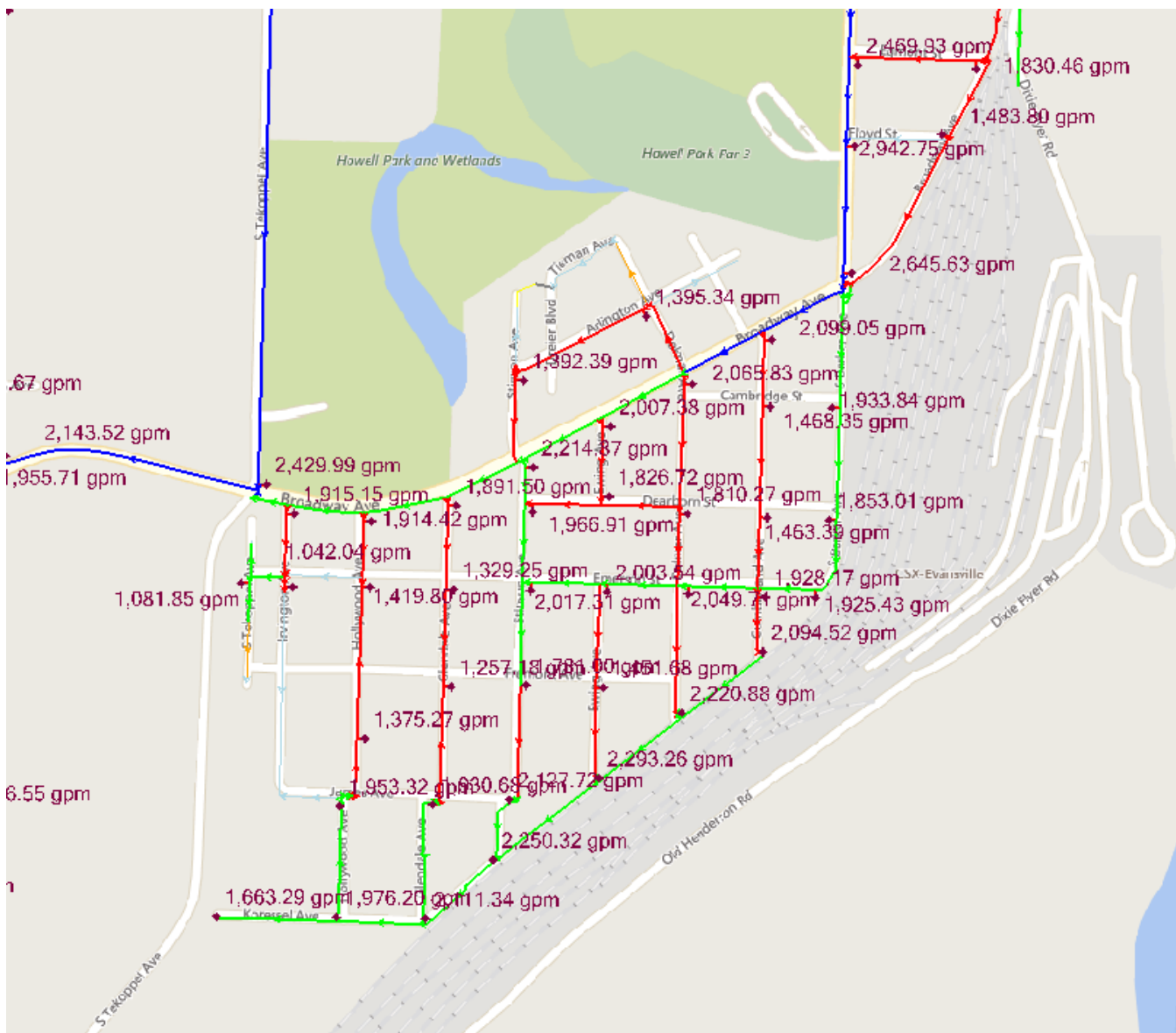
Figure 2. Existing Available Fire Flow
