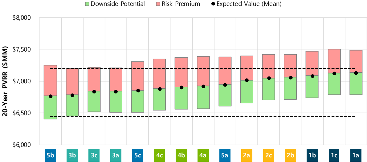
Figure 8.38 | PVRR Range, Scenario C: Carbon Tax + Low Gas + Low Load ($MM)
