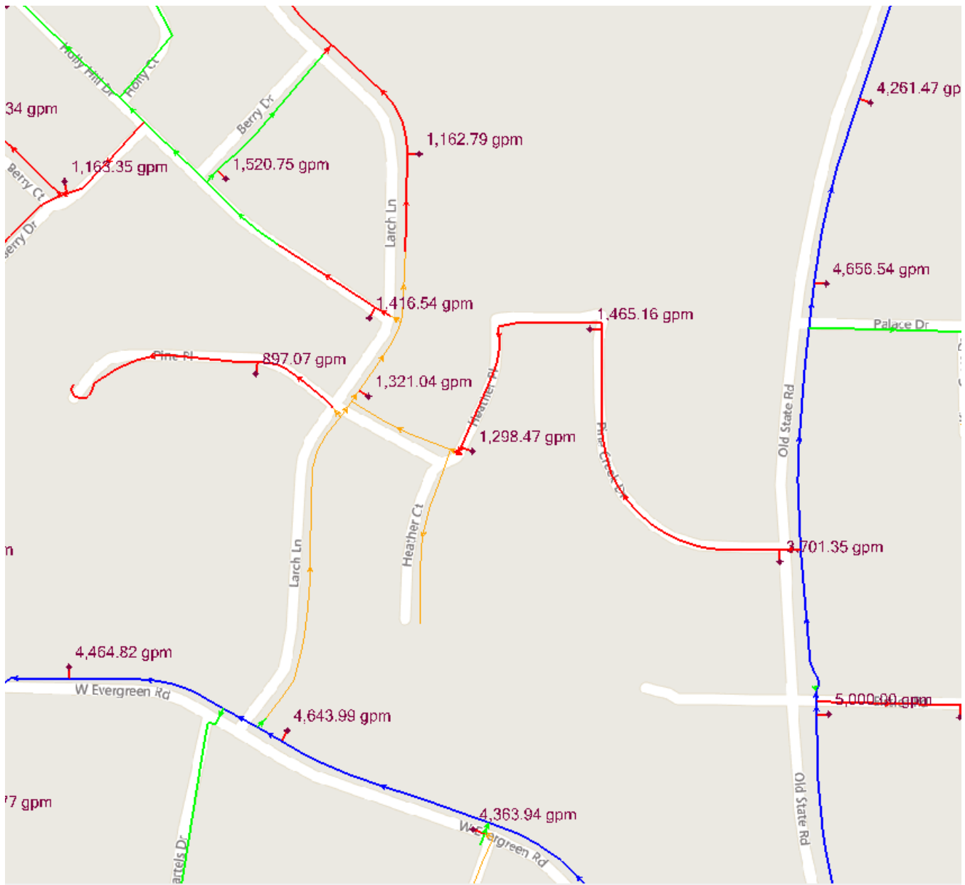
Figure 2. Existing Available Fire Flow
