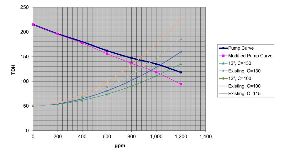
I:\Azure\UTILI\210623-Twin Lakes Pigging\00-Design-Construction\06-Calcs-Basis of Design-Hydraulics-Process Control-Equip\Hydraulics\PS Hydraulics ver 21 MJK - All 12 repaired Full Speed Chart 1 of 1 9/8/20219:35 PM
