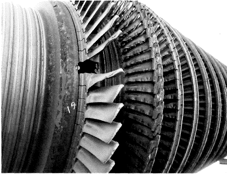
Photograph 7, Missing Blade STG HP Section
