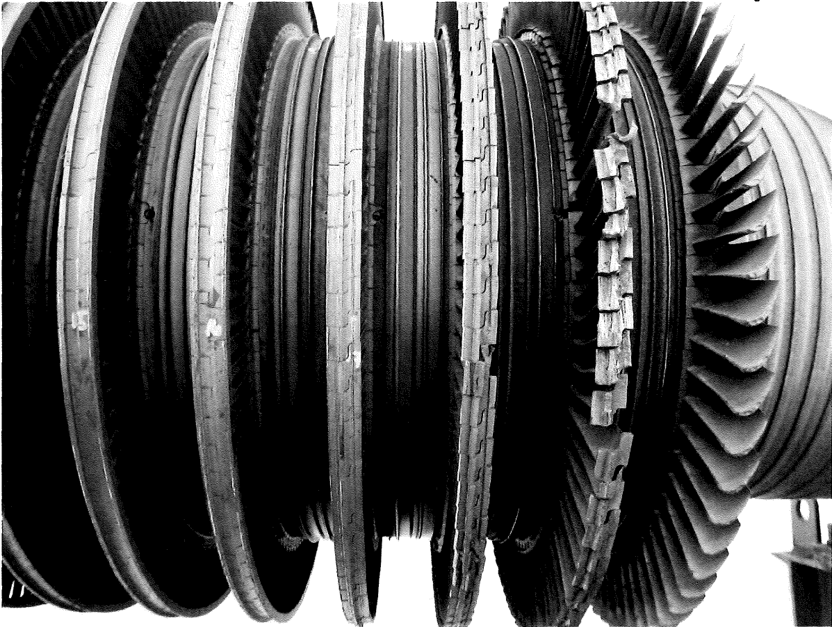
Photograph 5, Damaged STG Turbine (HP section)
