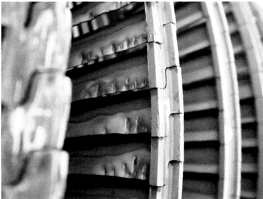
Photograph 6, Damaged STG Blade Edges
